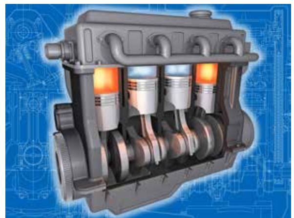
Figure 9: Combustion engine simulation for the calculation of elasto-hydrodynamic pressure.
